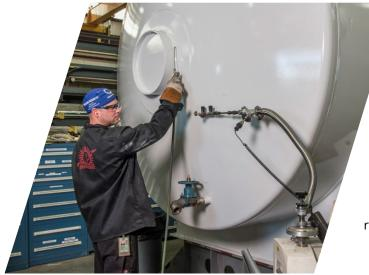
Like all of our equipment, these hydrogen transport and storage tanks are ruggedly built, ensuring peak performance under virtually all environmental conditions throughout the world. The tanks are built with Type 304 stainless steel internally and high-strength carbon steel externally, with designs customized to meet a wide variety of specifications.
